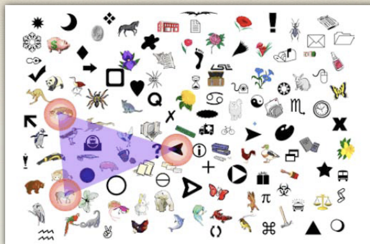
* Example where a user recognizes three objects and click inside the triangle defined by the objects
